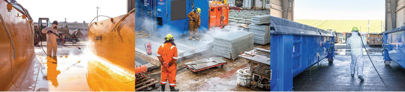
Hydroblasting (up to  $\leq 40,000$  psi), also known as water blasting or high-pressure water jetting, is an industrial cleaning method that uses a high-pressure stream of water to clean surfaces and remove unwanted substances. Our 3D cleaning method avoids the use of harsh chemicals, while effectively preparing and cleaning surfaces of tanks and pipelines, and cleaning drainage systems. This method avoids the need for confined space entry.
